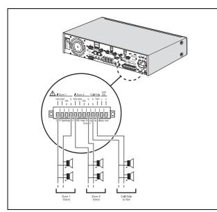
figure 4.8: Connecting speakers
